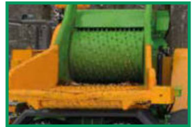
Aggressive Anpressrolle Ø 800 mm
